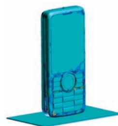
**Figure 1.13:** Virtual drop tests of a cell phone are performed using Abaqus to analyze the stress and strain of main parts as the phone strikes a surface from various directions. Realistic simulation enables design engineers to evaluate whether the stiffness of the phone's components meets performance requirements. (Image courtesy of Lenovo)
