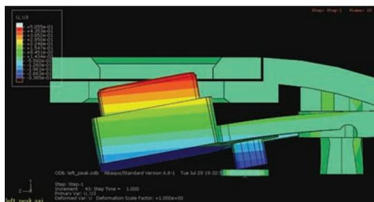
**Figure 1.12:** A process simulation for a notebook power button is performed using Abaqus to analyze the stress caused when pushed. Realistic simulation enables design engineers to evaluate whether the notebook's power button meets performance requirements. (Image courtesy of ASUSTeK Computer, Inc.)
