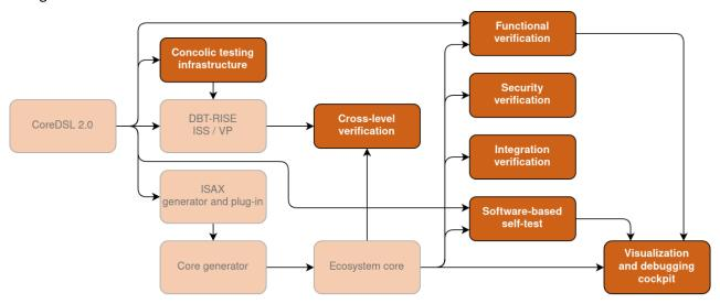
Figure 1: The Scale4Edge Hardware Verification Ecosystem
