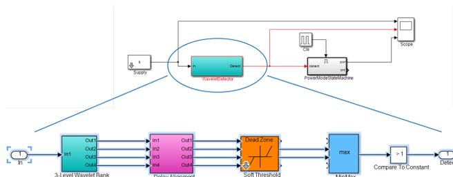
Fig. 6. Example Simulink model of the entire design concept of a power quality aware analog/mixed-signal power device
