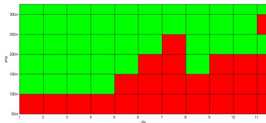
Fig. 9. Hardware performance evaluation on a microcontroller platform for a supply line disturbed by a short-term transient sinusoidal overlay (disturbing signal amplitude (V) versus signal frequency (kHz))
