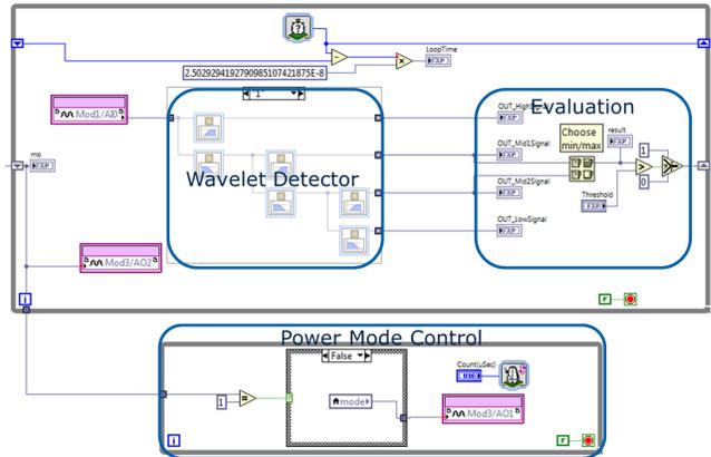
Fig. 8. Wavelet-based detection scheme for automotive supply line disturbances implemented and deployed on a FPGA platform
