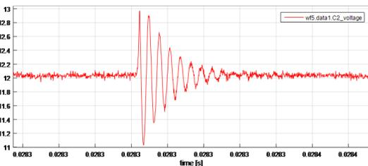
Fig. 4. Detail of short-term transient showing oscillatory shape on the power supply line
