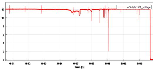
Fig. 3. Recorded time series of supply line disturbances occurring on the automotive board net with transient faults prior to failure
