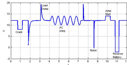
Fig. 1. ISO7637-2 and main surges on automotive power net representing supply line disturbances for analog and mixed-signal power devices
