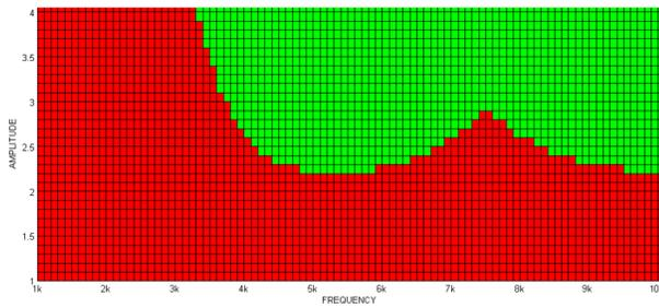
Fig. 10. Hardware performance evaluation on a FPGA platform for a supply line disturbed by a short-term transient sinusoidal overlay (disturbing signal amplitude (V) versus signal frequency (kHz))
