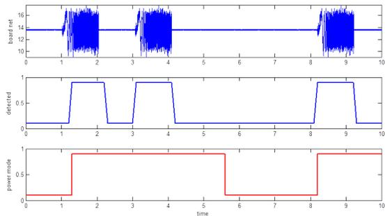
Fig. 7. Simulation results of wavelet-based detection scheme for supply line disturbances (top trace) with power mode reaction (lower trace) using Simulink model
