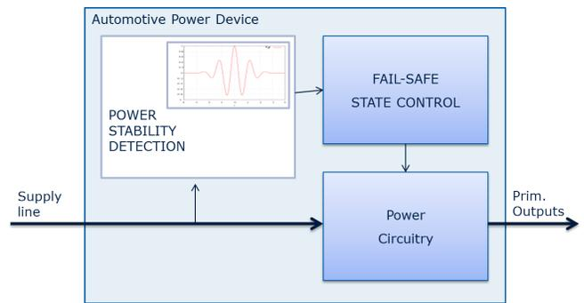
Fig. 5. Concept of automotive smart-power device incorporating embedded wavelet-based detection scheme for supply line disturbance and fault detection
